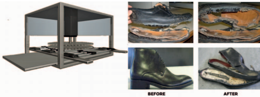
Figure 2 : Automatic disassembly of shoes using specially design cutting operation
