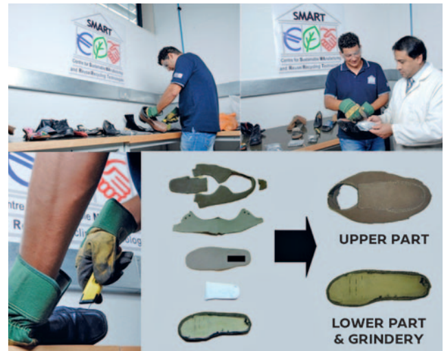
Figure 1 : Manual disassembly of shoes for component reuse and/or material separation.
