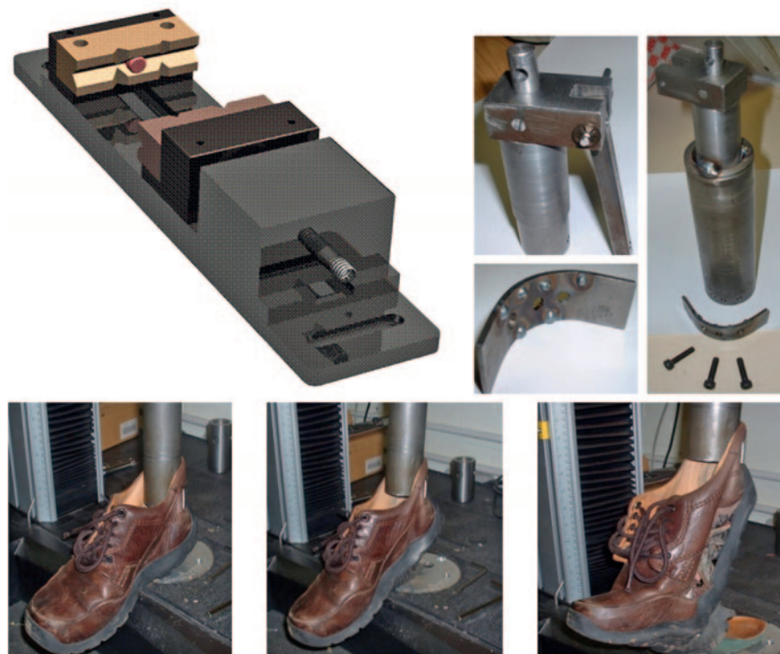
Figure 3 : Automatic disassembly of shoes by using specially design tools and fixtures.
